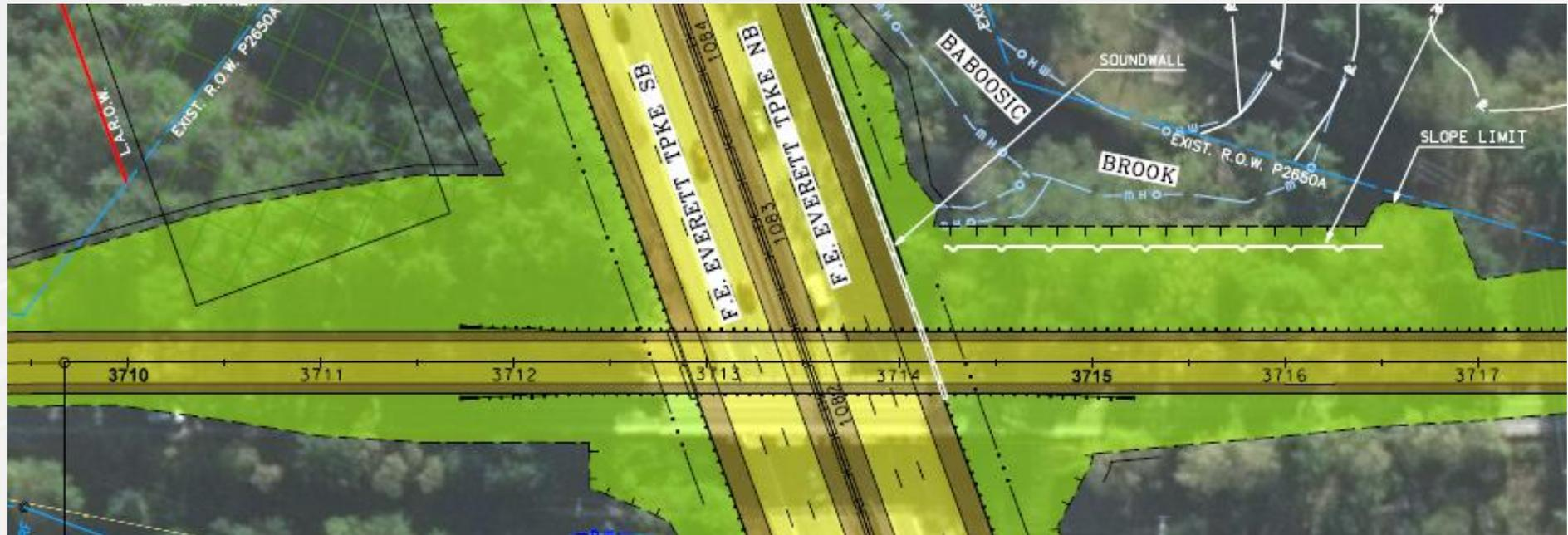
Wire Road: New bridge to be built to the north, while maintaining one way alternating traffic on existing bridge.
